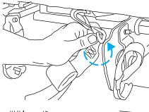
5. Clip the tether strap to the seat tether slot bracket at the lower rear portion of the seatback.
